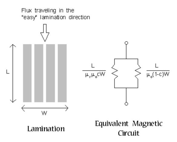
Figure A.5: Equivalent circuit for flux in the "easy" direction
