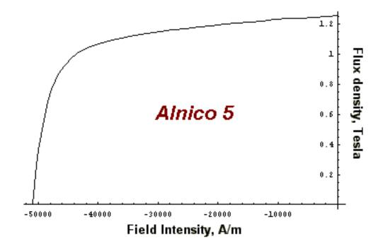
Figure A.1: Sample demagnetization curve for Alnico 5
