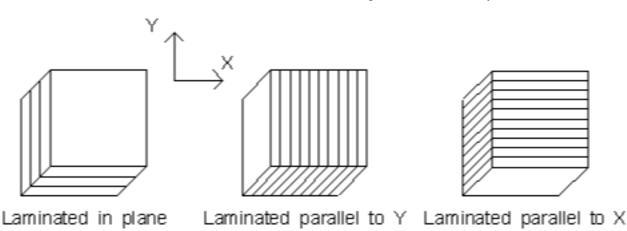
Figure 2.12: Different lamination orientation options.
