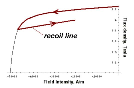
Figure A.4: Recoil in partially demagnetized Alnico 5.
