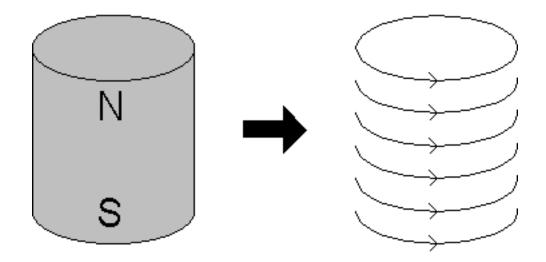
Figure A.2: Magnet as an equivalent current sheet.
