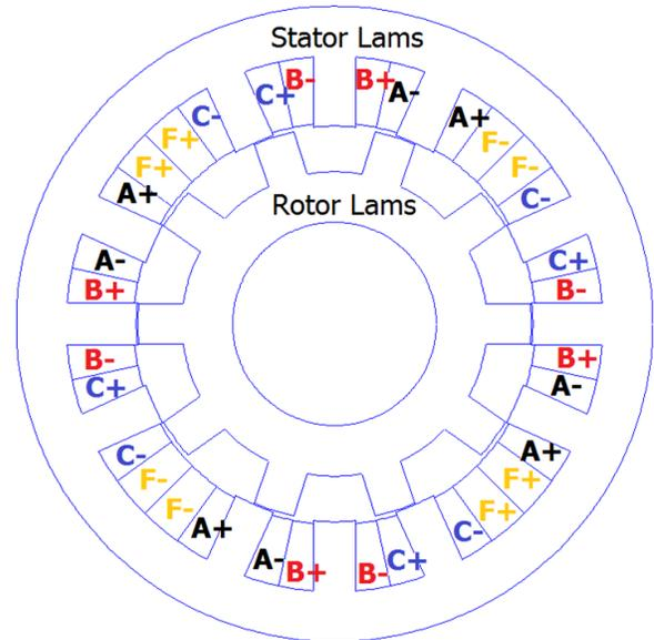
Fig. 1. Cross-section of a Doubly Salient Synchronous Machine.
