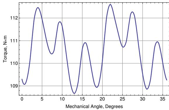
Fig. 8. Torque vs rotor angle for 110N\*m/4kRPM (U).
