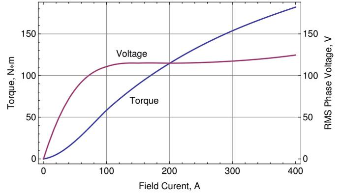
Fig. 3. Phase Voltage versus Field Current for a typical machine (at a  $60^\circ$  phase angle)
