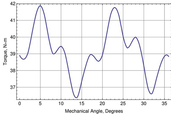
Fig. 9. Torque vs rotor angle for 39N\*m/12kRPM (F).
