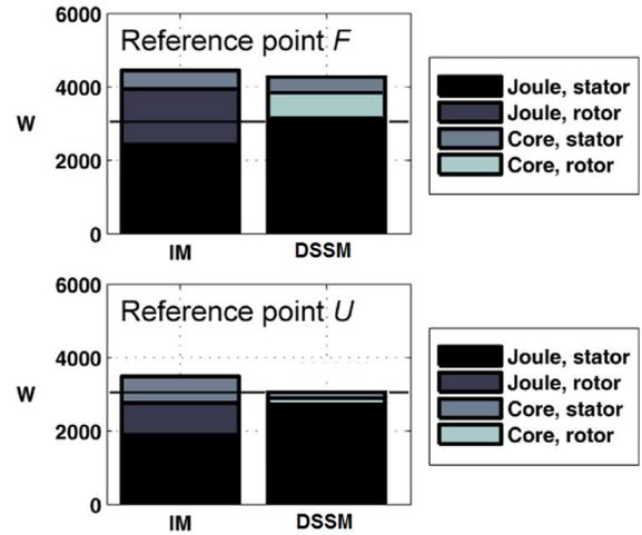
Fig. 7. Losses at 110N\*m/4kRPM (U) and 39N\*m/12kRPM (F).
