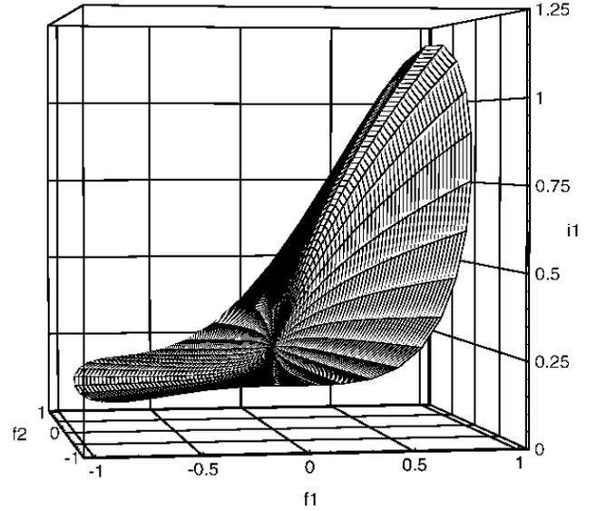
Figure 4: Eight pole power optimal force-to-current mapping.
