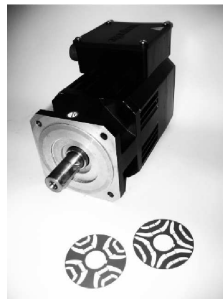
(a) IPM rotor with tangentially magnetized PMs, (b) an IPM motor and laminations with radially magnetized PMs.
