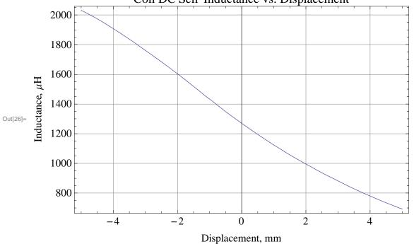
Coil DC Self Inductance vs. Displacement
